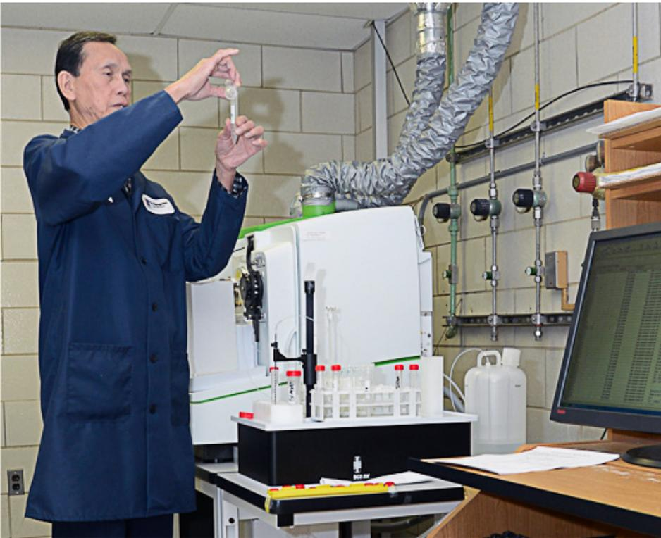
**Chemist Lito Chiu prepares a sample for metal analysis at the South Durham Water Reclamation Facility.**
