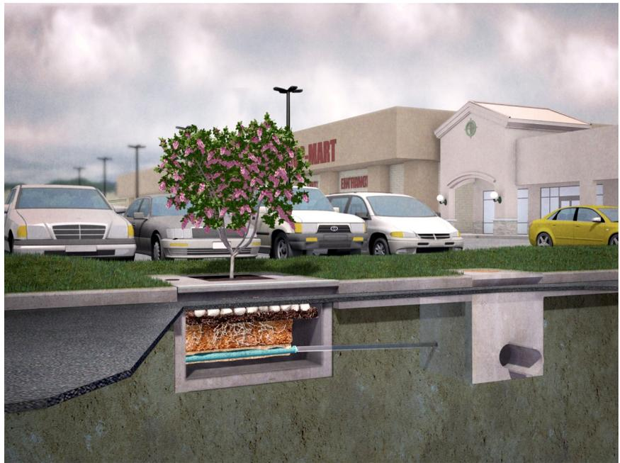
*A Filterra bioretention box removes pollution from stormwater runoff as it enters the drainage system.*
