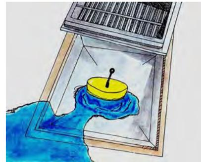
You can contain wastewater with storm drain mats (left), flexible berms (middle) and flexible or inflatable drain plugs (right). If you use this containment method, you will need to wash down the pavement when you are done and collect that water as well.
