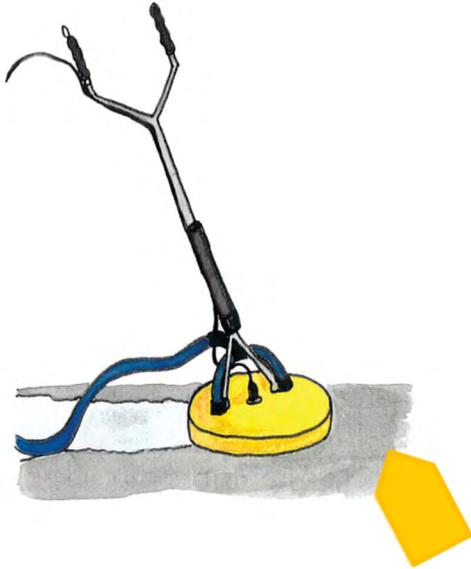
Some rotary cleaners also collect dirty wash water along with supplying high pressure water for cleaning. This water is carried through a hose to a storage tank.
