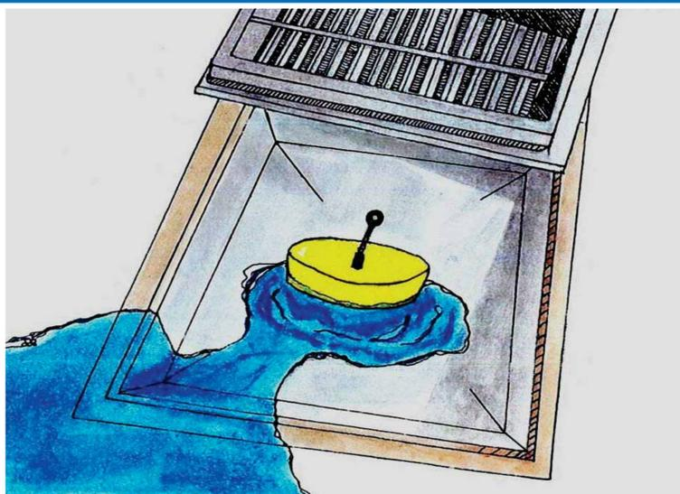
Drain plugs can be used to collect then contain water in drop inlets
