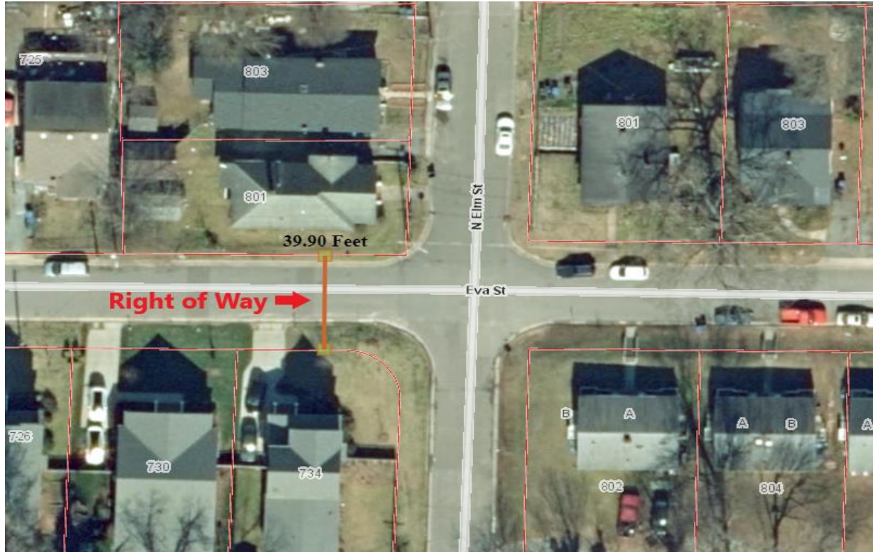
Fig 2. Cross Street at Eva Street and North Elm Street in East Durham (Durham Go Maps). Note how the Right-of-Way varies greatly between the North side of Eva street vs the South side of Eva street. In this case street trees would not be planted on the North Side of the street because the Right-of-Way starts and ends at the curb.
