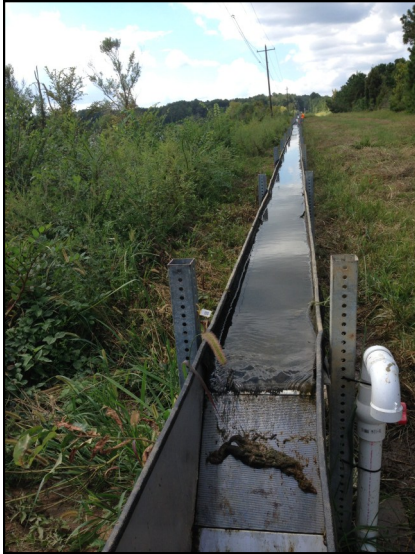
Twenty gallons of lake water per minute flow through this device to grow algae and remove nutrients from the water.
